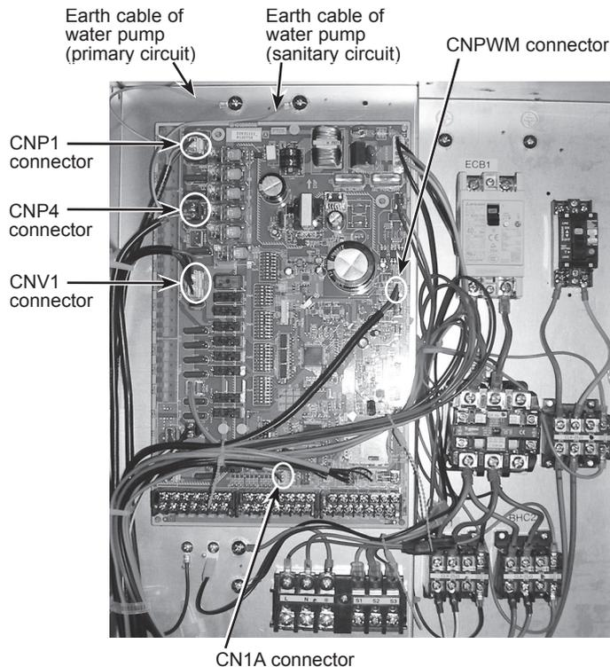
\* The photos shown are of the EHST20C-VM6C model with optional immersion heater.
