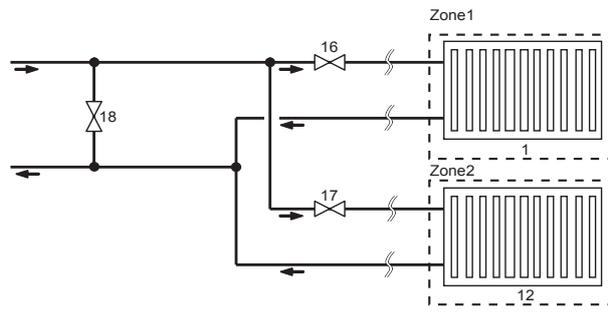
1. Zone1 heat emitters (e.g. radiator, fan coil unit) (local supply)
