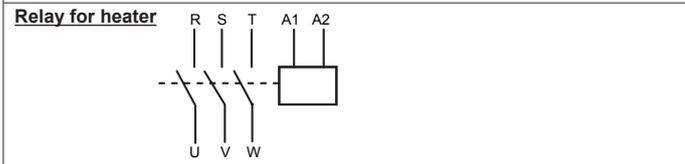
When the applied voltage is not 230V AC across the terminals A1-A2, check the terminals R-U, S-V, and T-W are open. When the applied voltage is 230V AC across the terminals A1-A2, check the terminals R-U, S-V, and T-W are short.
