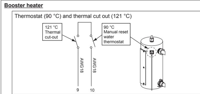
Measure the resistance between the terminals with a tester.
