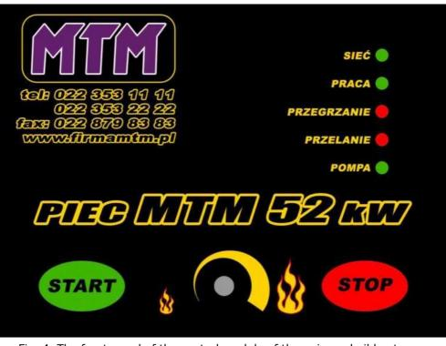
Fig. 4. The front panel of the control module of the universal oil heater.
