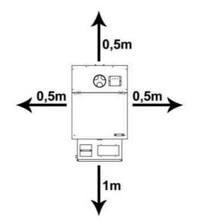
Fig. 2. Minimal safety space around the device.
