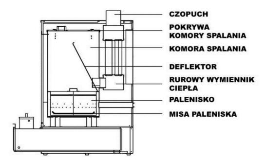
Fig. 3. Combustion chamber structure [Flue], [Chamber cover], [Chamber], [Deflector], [Pipe exchanger], [Furnace], [Furnance Bowl]
