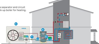
Basic scheme. It does not include filters, automatic air vents, expansion vessels, shut-off valves, check or safety valves present in any installation
