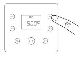
Change the temperature setpoint using the following buttons  $\bigwedge$  and  $\bigvee$
