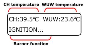
The burner may work in three working modes ("STOP", "IGNITION", "AUTOMATIC WORK"). The mode changes when the "MODE/\to " button is pressed. Activating the "STOP" mode is possible in all modes after pressing the "MODE/\to " button for 3 seconds. When Stop is activated, the burner goes at "Burning off" process (if there is fire) and the at "Cleaning" process.
