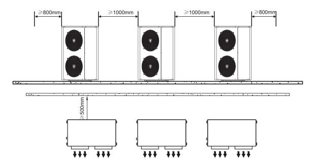
Attention: Please make sure that the height of other stacked thing around the heat pump should lower than our heat pump, and please keep distance between these two parts.
