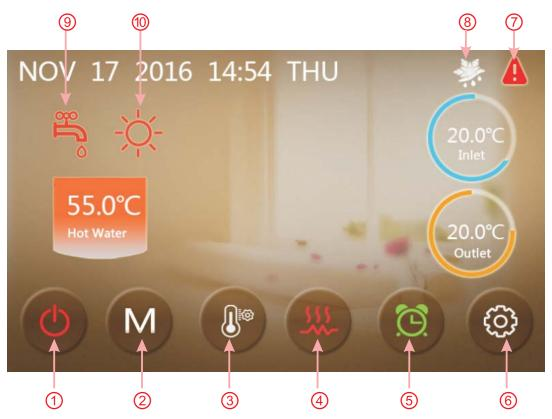
Remark: the wire controller can display the temperature unit as "°F" or "°C" according to the unit model you bought.
