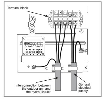
figure 32 - Connections to sinlge phase outdoor unit's terminal block
