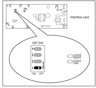
figure 22 - Location of DIP switches and diodes on the hydraulic unit interface card
