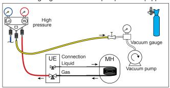
Create a vacuum until the residual pressure\* in the circuit falls below the value given in the following table.
