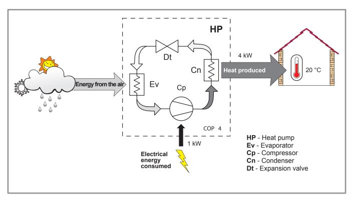
figure 8 - Heat pump operating principle
