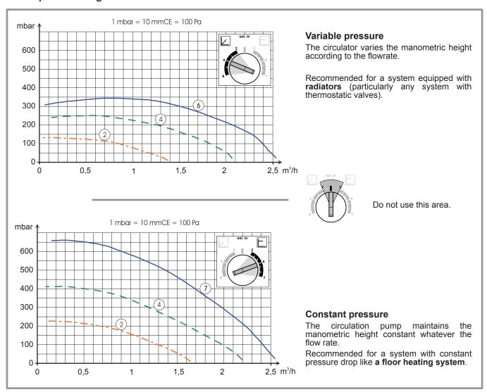
figure 28 - Hydraulic pressures and flow rates available
