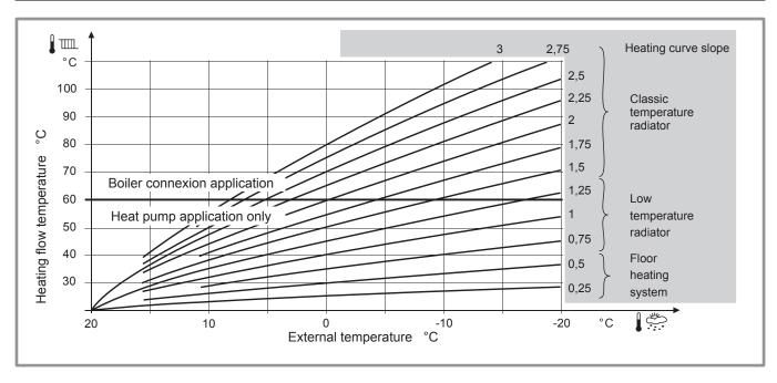
figure 44 - Heating curve slope (line 720)
