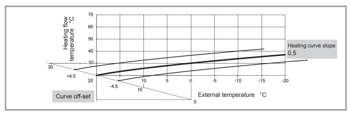
figure 45 - Off-set of the heating curve (line 721)
