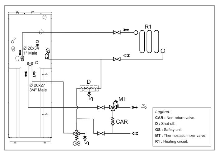
figure 23 - Overall hydraulic layout
