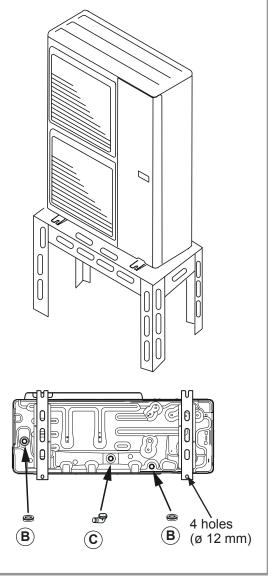
figure 12 - Positioning of the outside unit, draining away the condensate
