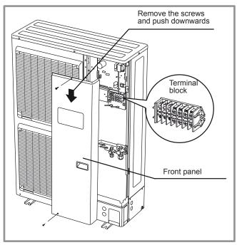
figure 34 - Access to 3-phase outdoor unit's terminal block
