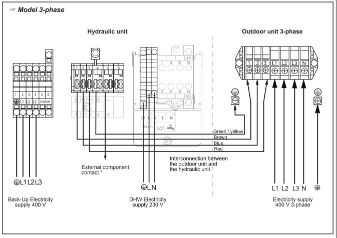
figure 41 - Connection to terminal block and power relays
