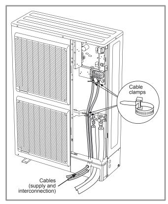
figure 36 - Finalisation of connection to 3-phase outdoor unit
