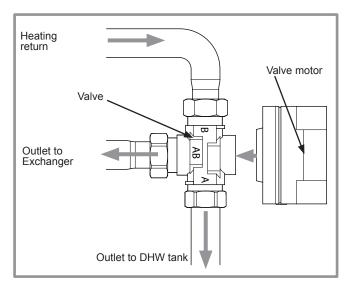
figure 56 - Fitting the distribution valve
