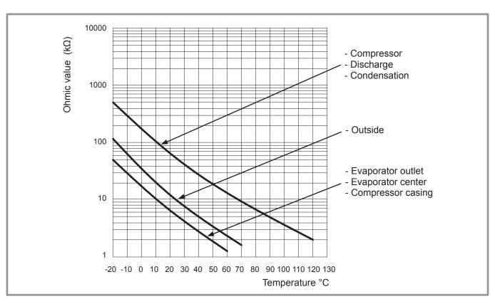
figure 5 - Ohmic values of the sensors (Outdoor unit)
