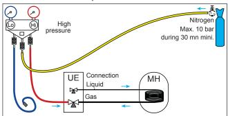
Search for leaks with a leak detector product, repair and repeat the test.
