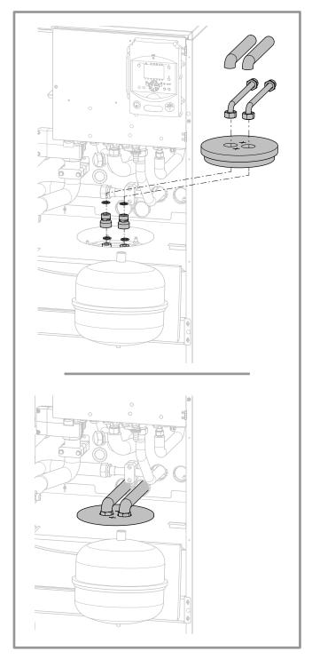
figure 24 - DHW pipes mounting
