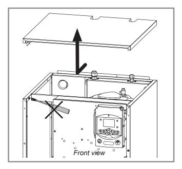
figure 15 - Removing the cover
