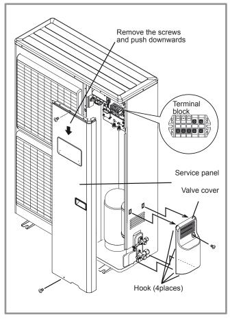
figure 31 - Access to sinlge phase outdoor unit's terminal block
