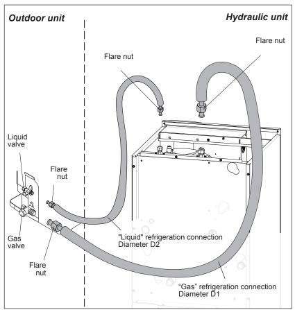
figure 19 - Connecting the flared connections (Pipe diameters and permissible lengths)
