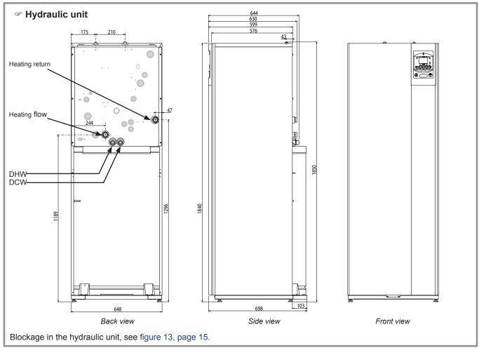
figure 2 - Dimensions in mm
