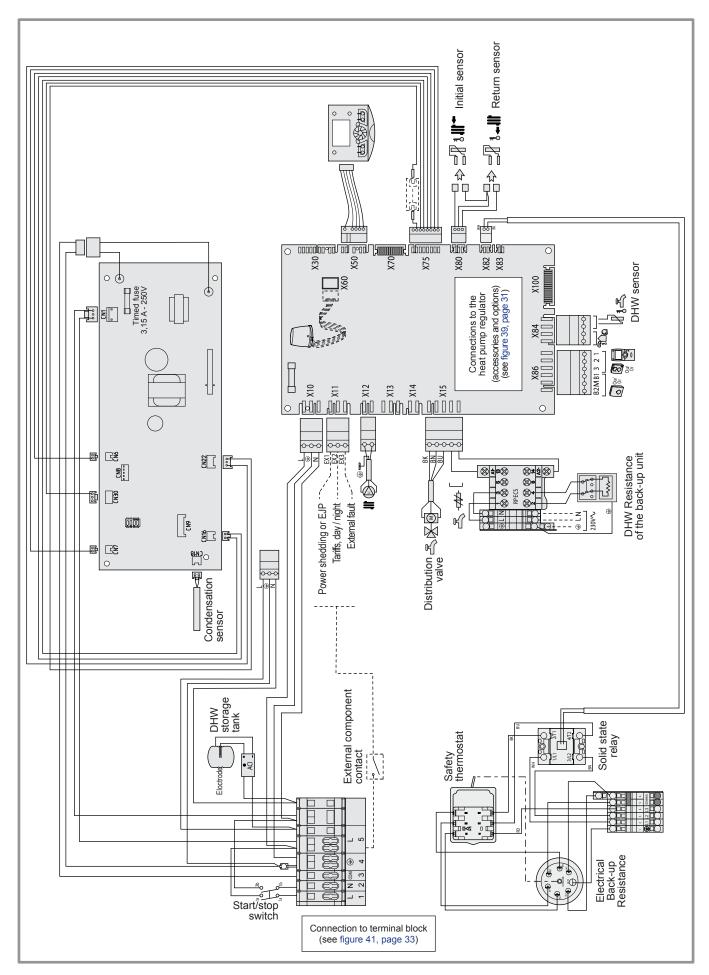
figure 51 - Electrical wiring, Hydraulic unit High Power integrated DHW 3-phase (Except installer's connections)
