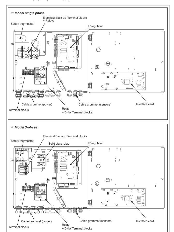
figure 40 - Access to hydraulic model electric box and description
