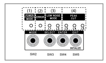
figure 54 - LED display on the 3-phase outdoor unit
