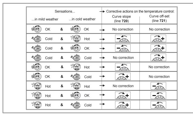
figure 46 - Corrective actions in the case of discomfort
