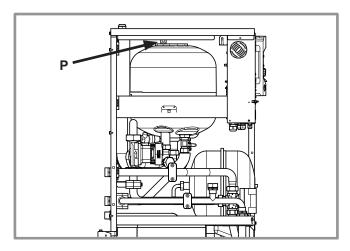
figure 26 - Hydraulic module bleeder valve
