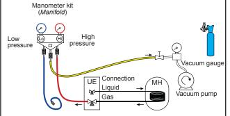
**b**) Stop the vacuum pump, close the valve end of the service hose (yellow). Connect the hose to the expansion valve of the nitrogen bottle, inject 2 bars, close the flexible hose valve,
