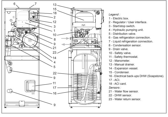
figure 7 - Hydraulic unit components
