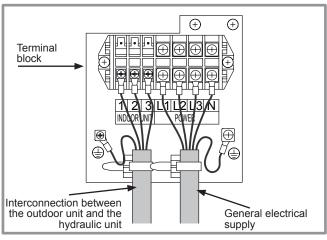
figure 35 - Connections to 3-phase outdoor unit's terminal block
