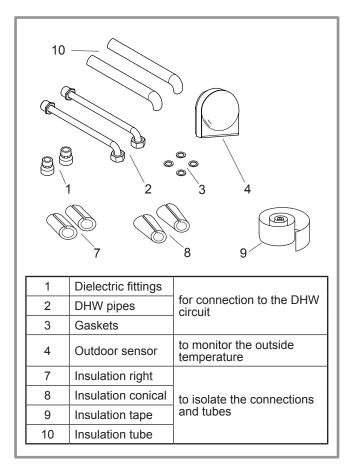
figure 10 - Accessories provided with the hydraulic unit
