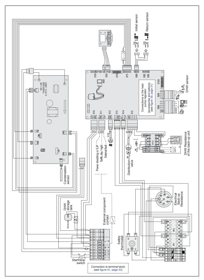
figure 50 - Electrical wiring, Hydraulic unit High Power integrated DHW single phase (Except installer's connections)
