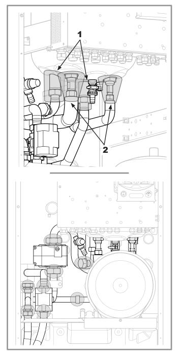
figure 27 - Thermal insulation
