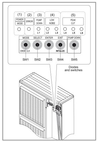
figure 52 - Location of switches and diodes on single phase outdoor unit
