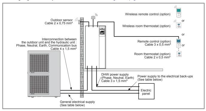
figure 30 - Overall layout of the electrical connections for a simple installation (1 heating circuit)
