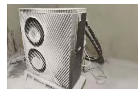
-25 °C Extremely Cold Test
