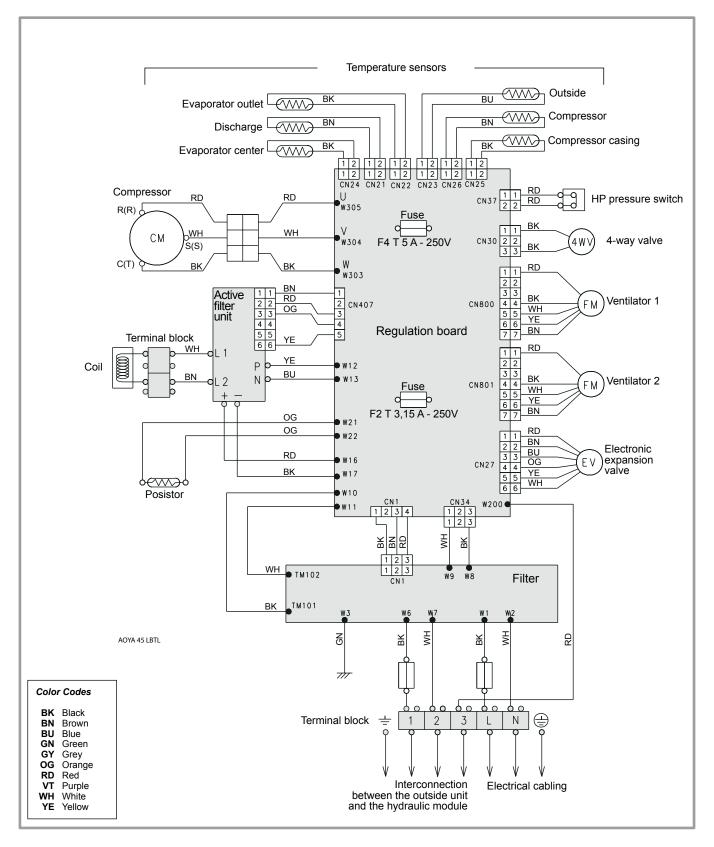
figure 38 - Electrical wiring of outside unit model extensa 13
