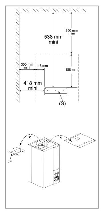
figure 14 - Mounting bracket
