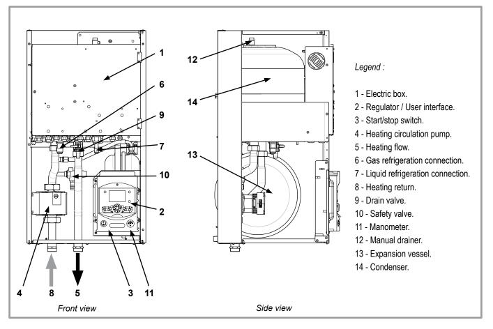
figure 8 - Hydraulic unit components
