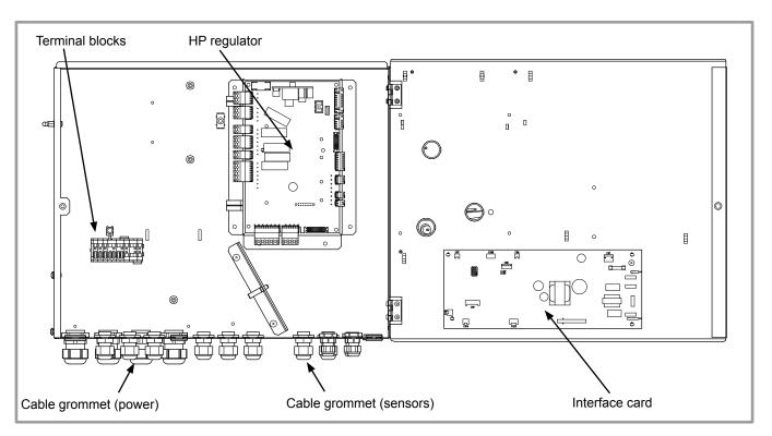
figure 26 - Access to hydraulic model electric box and description
