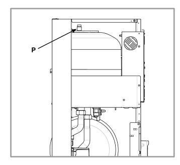
figure 19 - Hydraulic module bleeder valve
