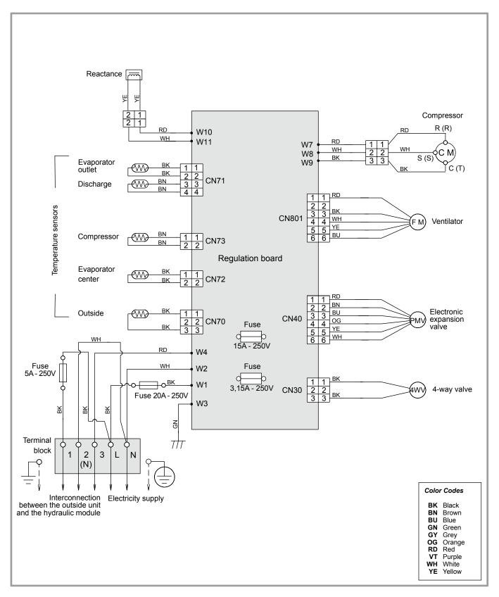
figure 36 - Electrical wiring of outside unit model extensa 5 & 6
