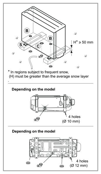
figure 13 - Positioning of the outside unit, draining away the condensate
