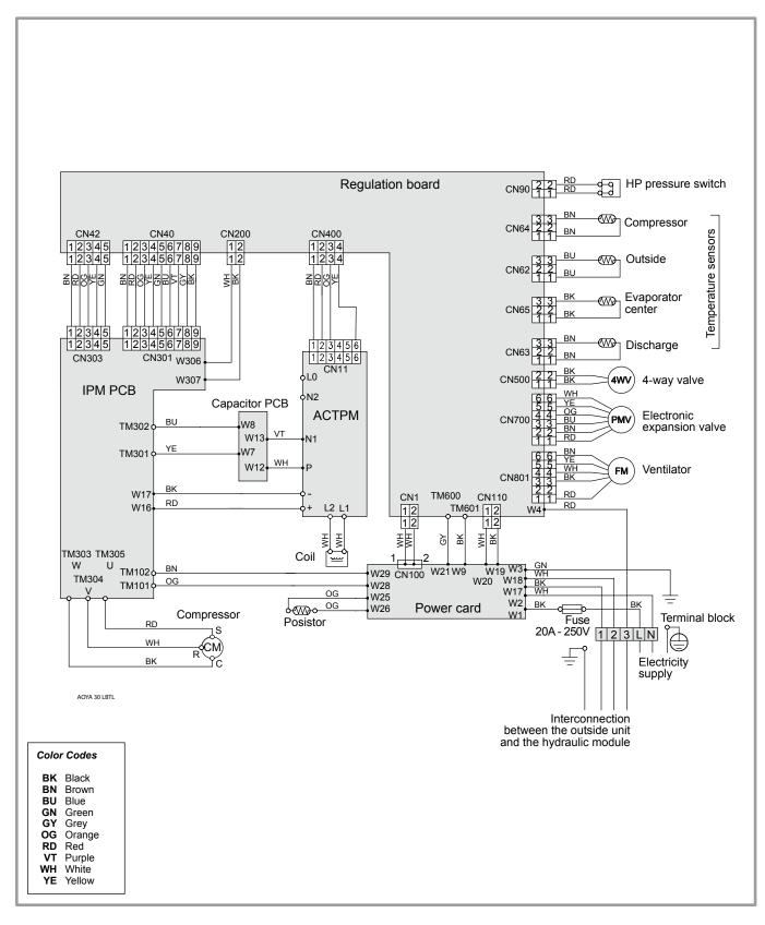
figure 37 - Electrical wiring of outside unit model extensa 8 & 10
