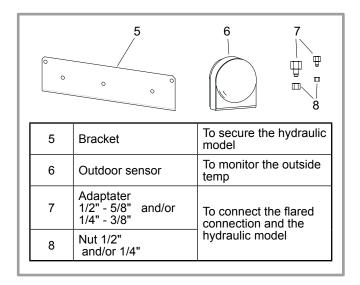
figure 11 - Accessories provided with the hydraulic unit
