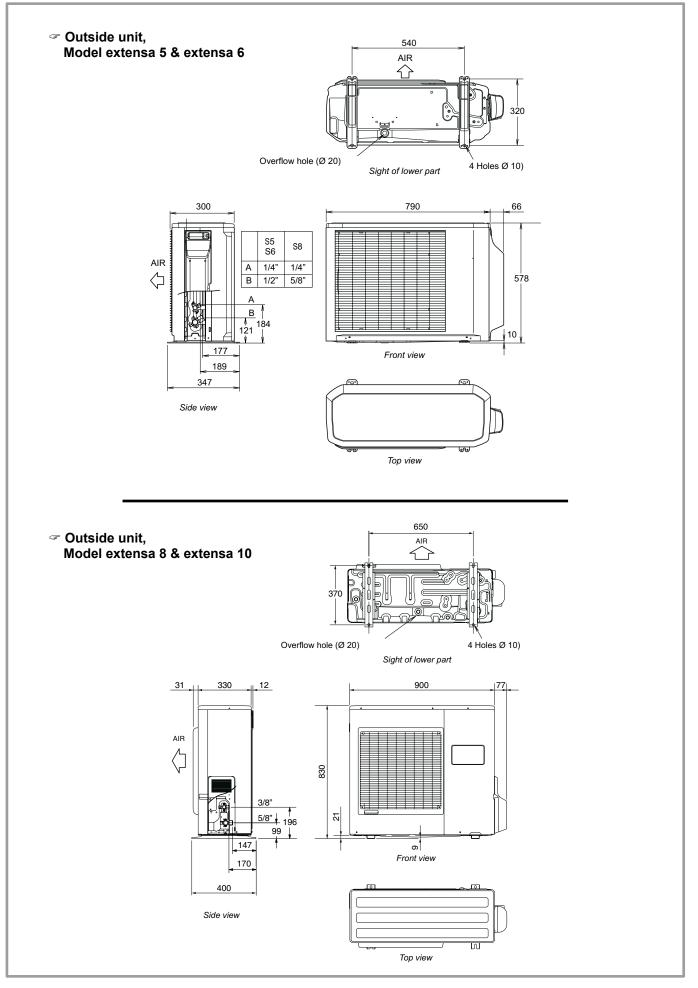
figure 1 - Dimensions in mm
