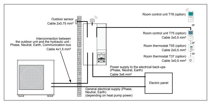
figure 22 - Overall layout of the electrical connections for a simple installation (1 heating circuit)
