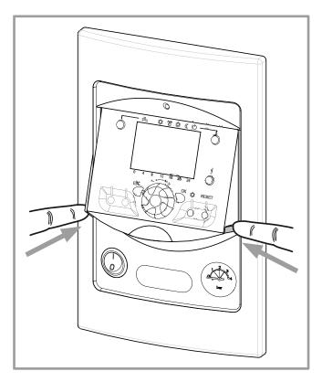
figure 31 - Closing the display
