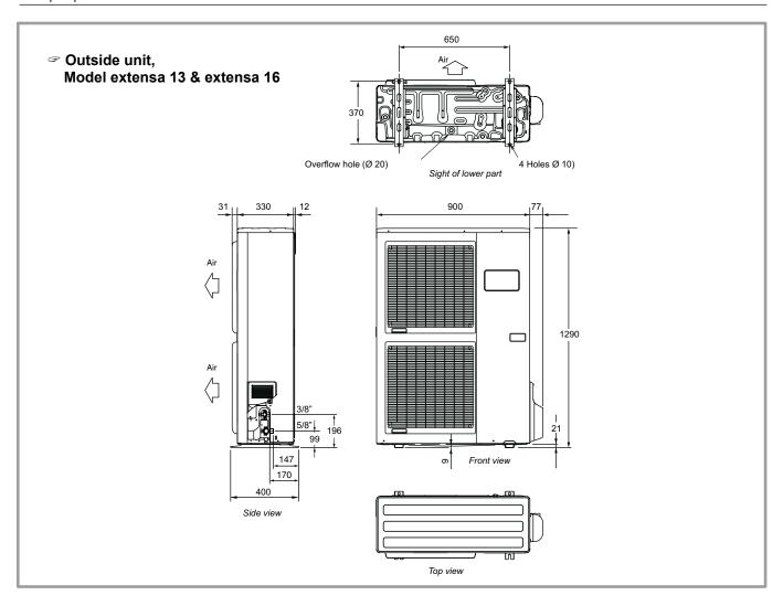
figure 2 - Dimensions in mm
