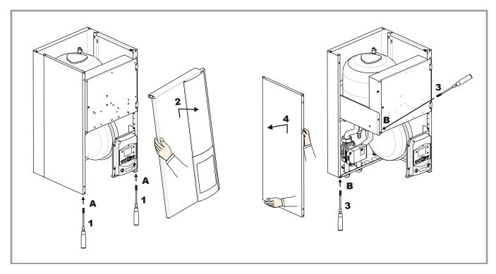
figure 15 - Removing the casing
