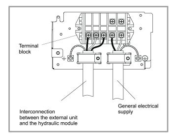
figure 24 - Connections to outside unit's terminal block
