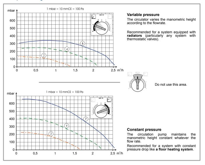
figure 21 - Hydraulic pressures and flow rates available
