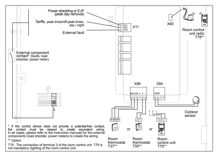
figure 28 - Connections to the heat pump regulator (accessories and options)
