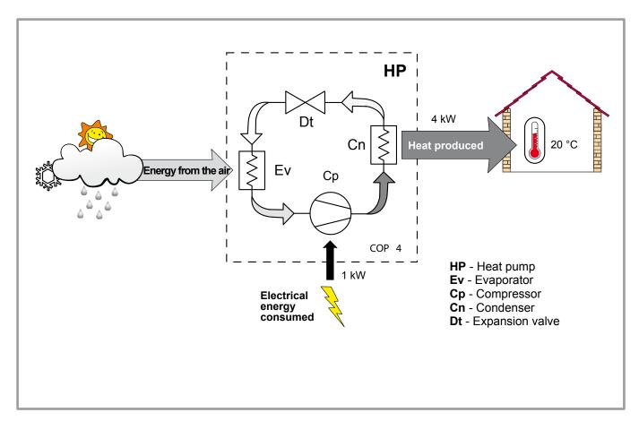
figure 9 - Heat pump operating principle
