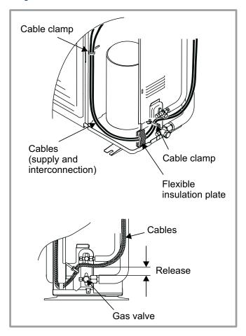
figure 25 - Finalisation of connection to outside unit
