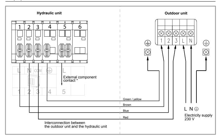
figure 27 - Connection to terminal block and power relays
