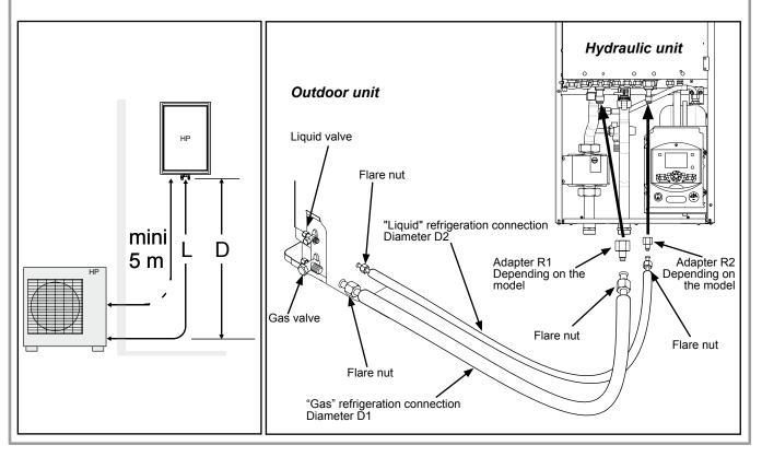
figure 16 - Connecting the flared connections (Pipe diameters and permissible lengths)
