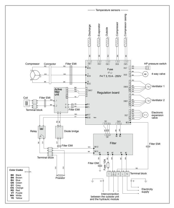
figure 39 - Electrical wiring of outside unit model extensa 16
