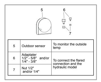
figure 10 - Accessories provided with the hydraulic unit
