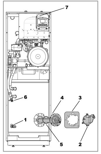
figure 40 - Emptying the hydraulic unit and/or Domestic hot water tank
