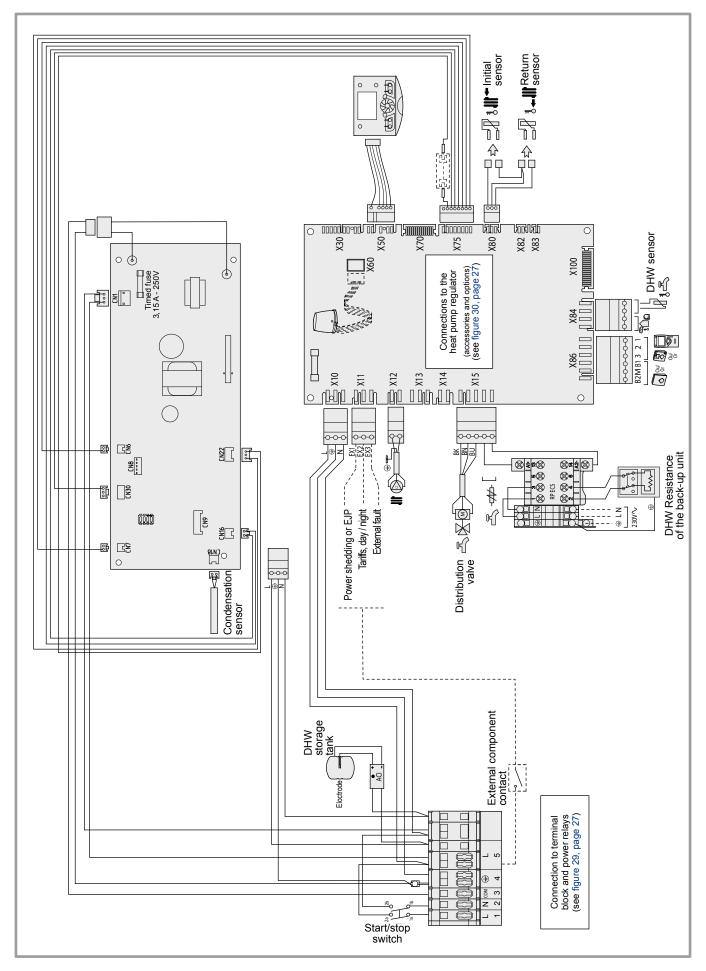
figure 39 - Electrical wiring, Hydraulic module (Except installer's connections)
