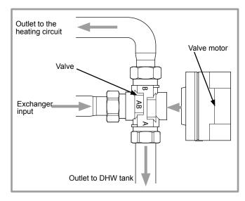
figure 41 - Fitting the distribution valve
