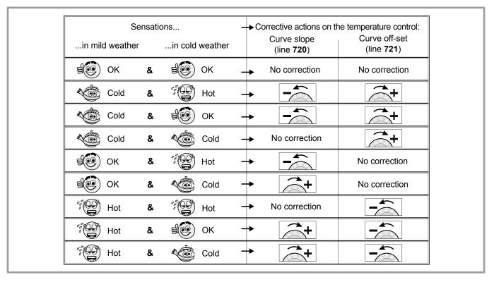
figure 35 - Corrective actions in the case of discomfort
