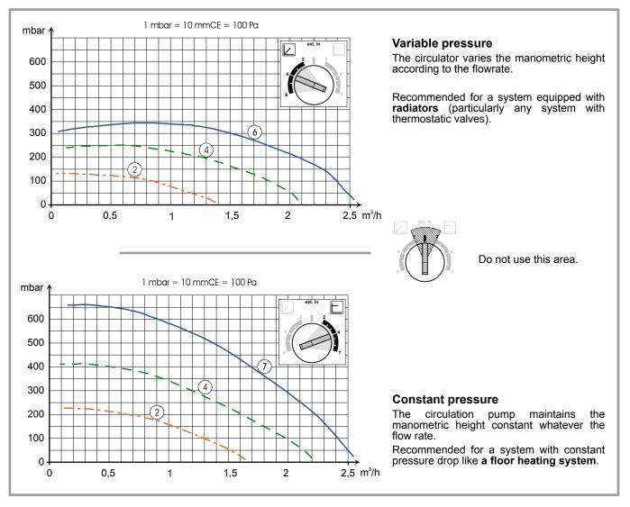
figure 23 - Hydraulic pressures and flow rates available
