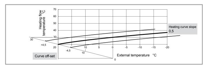
figure 34 - Off-set of the heating curve (line 721)
