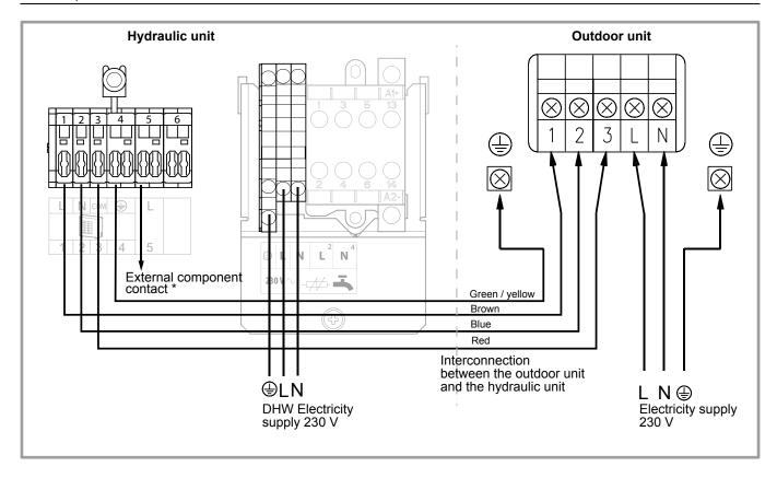
figure 29 - Connection to terminal block and power relays
