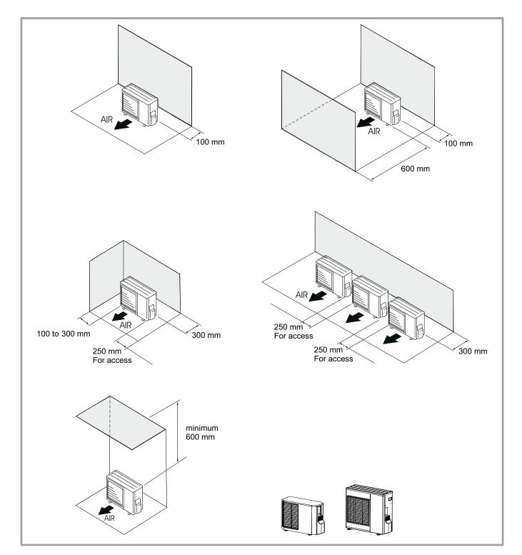
figure 11 - Minimum installation clearances around outside unit (all models)
