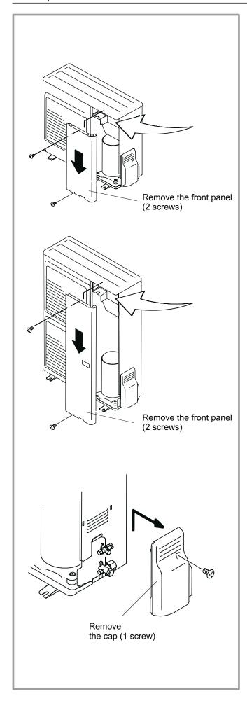
figure 25 - Access to outside unit's terminal block
