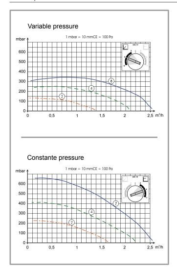
figure 3 - Hydraulic pressures and flow rates available
