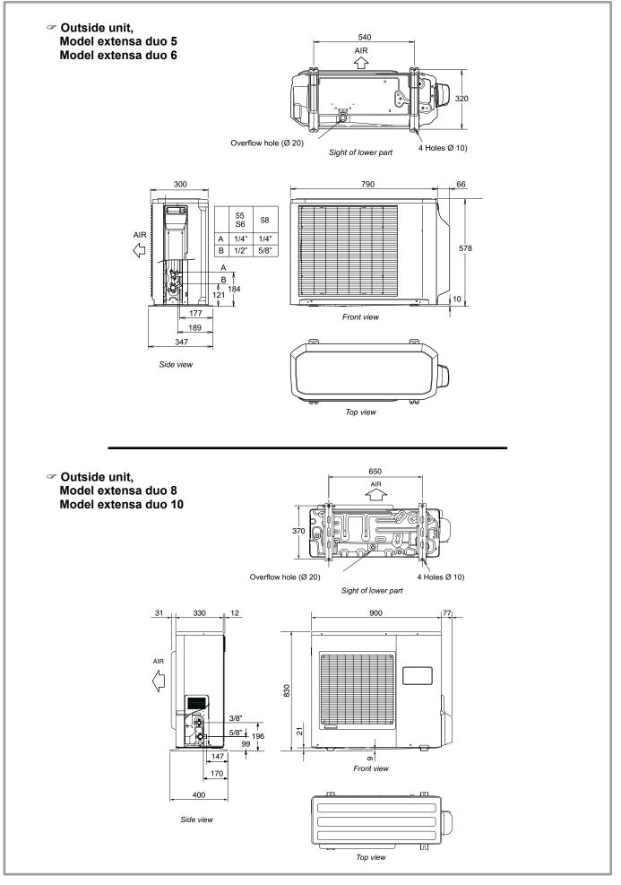
figure 1 - Dimensions in mm
