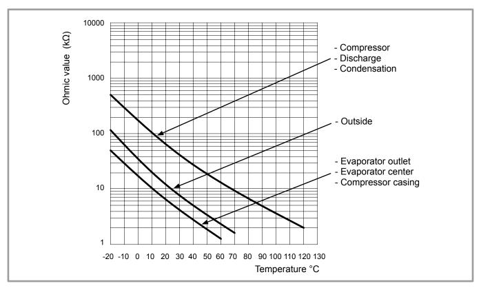
figure 5 - Ohmic values of the sensors (outside unit)
