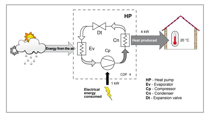
figure 8 - Heat pump operating principle
