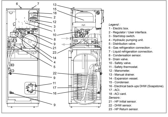
figure 7 - Hydraulic unit components
