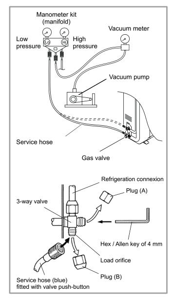
figure 18 - Extraction under vacuum and gassing
