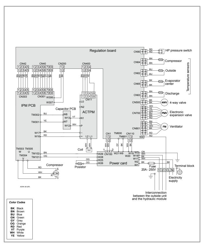
figure 38 - Electrical wiring of outside unit model extensa duo 8 & 10
