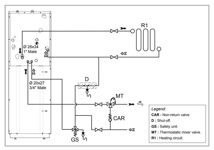
figure 19 - Overall hydraulic layout
