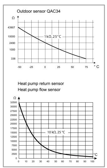
figure 4 - Ohmic values of the sensors (Hydraulic module)
