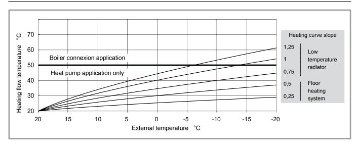
figure 33 - Heating curve slope (line 720)
