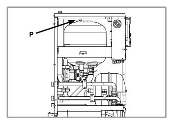
figure 21 - Hydraulic module bleeder valve
