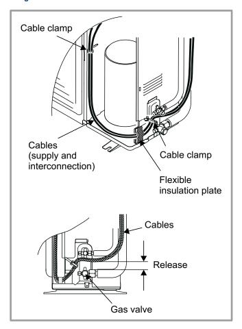
figure 27 - Finalisation of connection to outside unit
