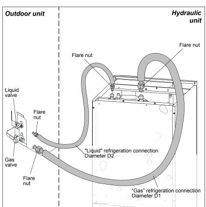
figure 16 - Connecting the flared connections (Pipe diameters and permissible lengths)
