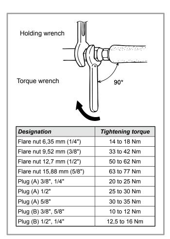
figure 17 - Tightening torque
