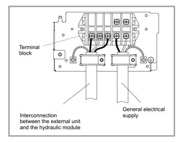
figure 26 - Connections to outside unit's terminal block
