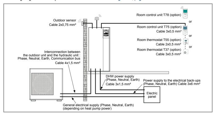
figure 24 - Overall layout of the electrical connections for a simple installation (1 heating circuit)
