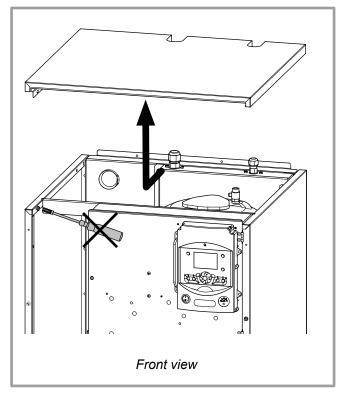
figure 14 - Removing the cover
