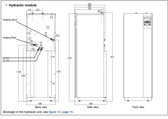
figure 2 - Dimensions in mm
