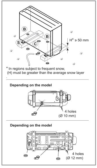
Figure 14 - Positioning of the outside unit, draining away the condensate
