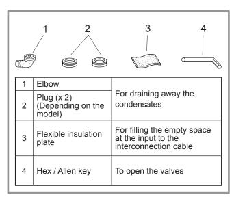
Figure 10 - Accessories provided with the outside unit
