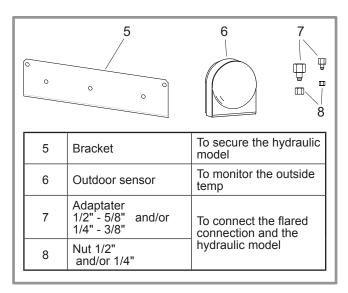
Figure 11 - Accessories provided with the hydraulic module
