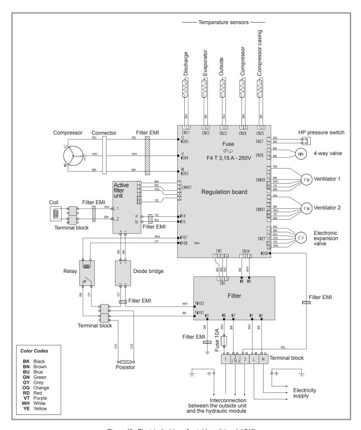
Figure 48 - Electrical wiring of outside unit (model S16)
