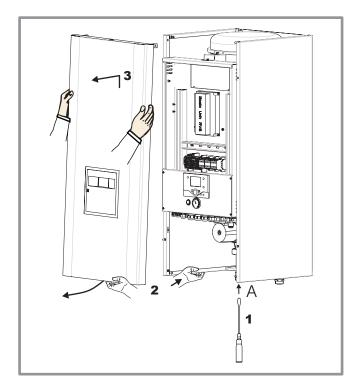
Figure 16 - Removing the front facing
