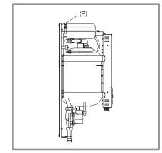
Figure 27 - Hydraulic module bleeder valve
