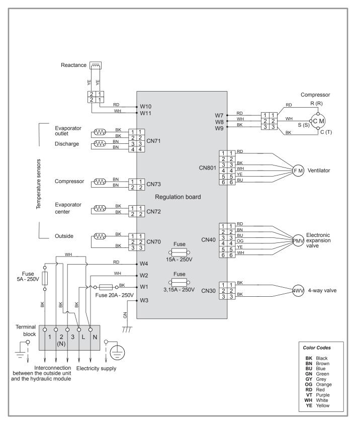
Figure 45 - Electrical wiring of outside unit (model S5, S6, S8)
