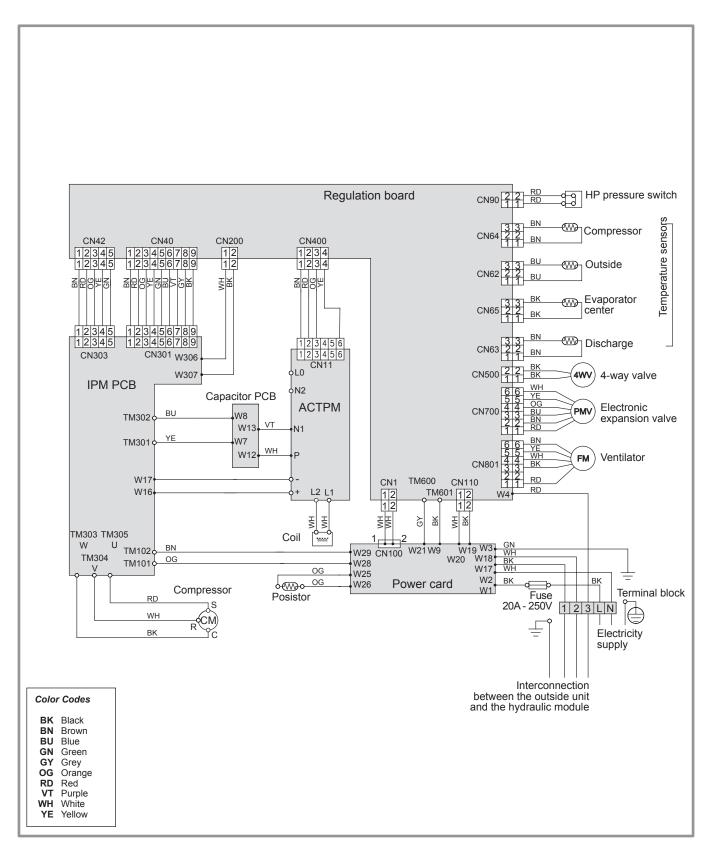
Figure 46 - Electrical wiring of outside unit (model S10)
