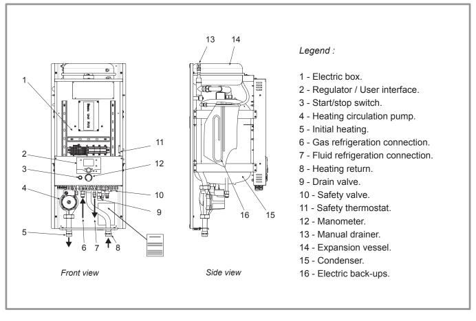
Figure 8 - Hydraulic module components
