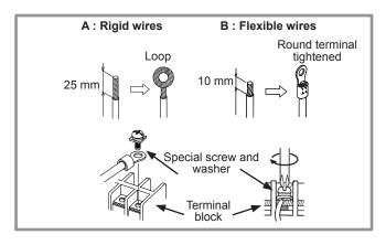
Figure 28 - Outside unit terminal block
