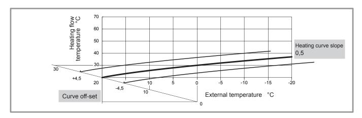
Figure 42 - Off-set of the heating curve (line 721)
