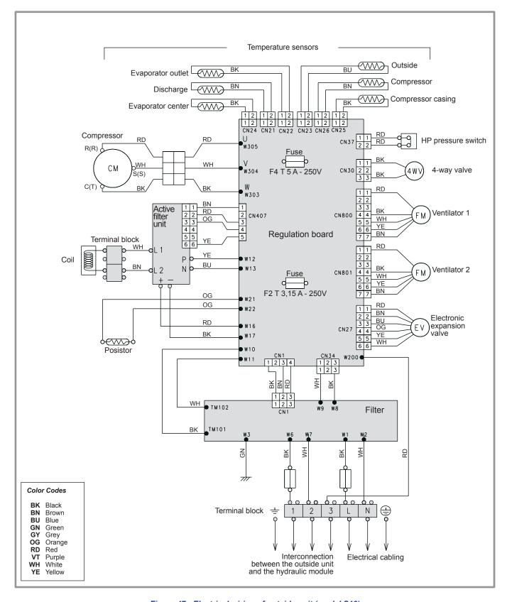
Figure 47 - Electrical wiring of outside unit (model S13)
