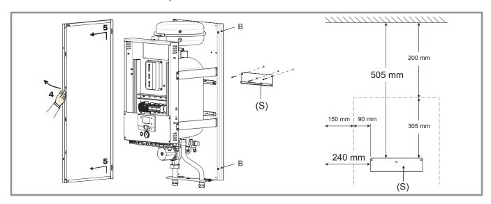
Figure 17 - Removing the sides and fixing the support (S)
