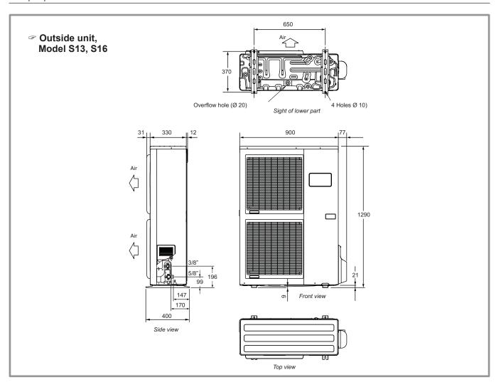
Figure 2 - Dimensions in mm
