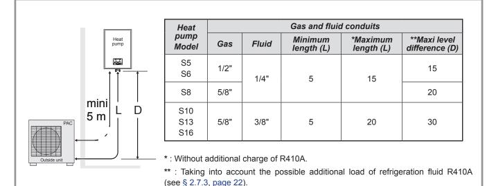
Figure 13 - Pipe diameters (in inches) and permissible lengths (in metres)
