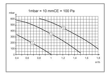
Figure 4 - Hydraulic pressures and flow rates available
