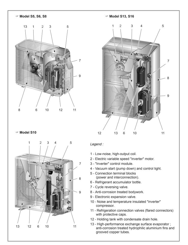
Figure 7 - Outside unit components
