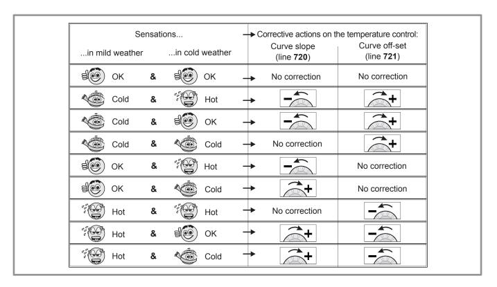
Figure 43 - Corrective actions in the case of discomfort
