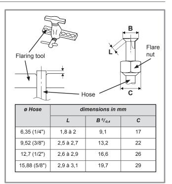
Figure 18 - Flaring for flare connections
