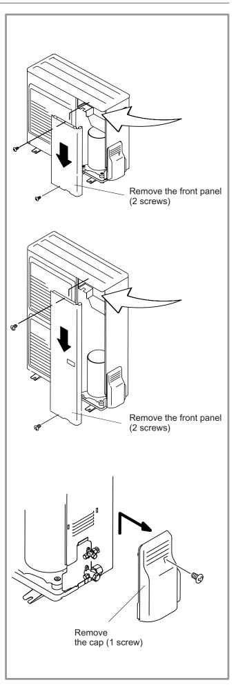
Figure 34 - Access to outside unit's terminal block (model S10, S13, S16)
