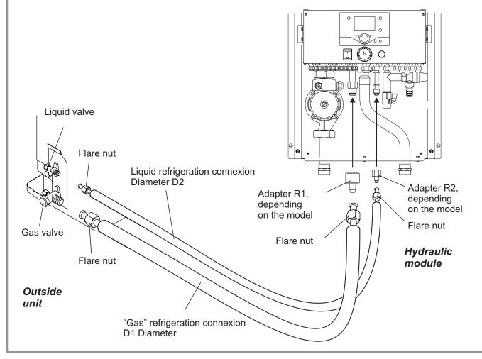
Figure 19 - Connecting the flared connections
