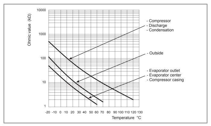
Figure 6 - Ohmic values of the sensors (outside unit)
