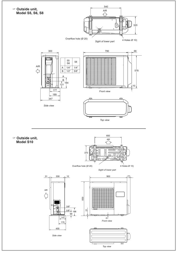
Figure 1 - Dimensions in mm
