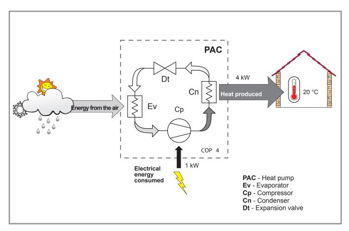
Figure 9 - Heat pump operating principle
