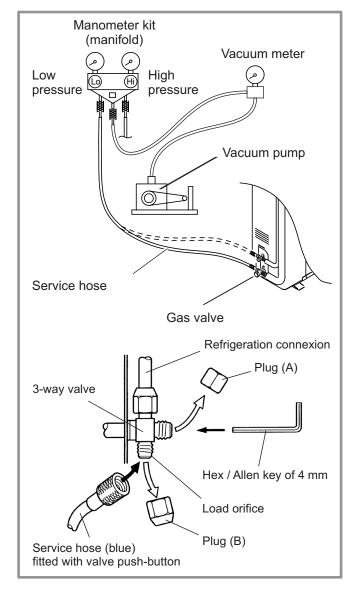
Figure 22 - Extraction under vacuum and gassing
