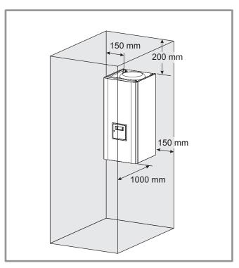
Figure 15 - Minimum installation clearances around the hydraulic module and distances to the combustible partitions
