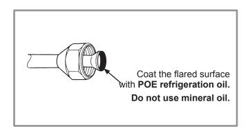
Figure 20 - Prevention of gas leaks
