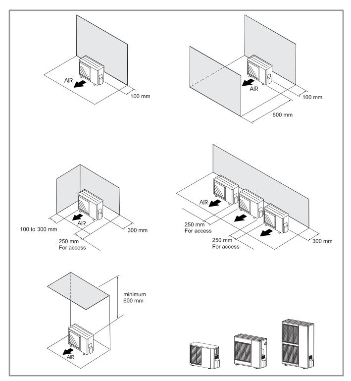
Figure 12 - Minimum installation clearances around outside unit (all models)
