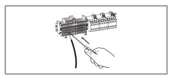
Figure 30 - Hydraulic module terminal block
