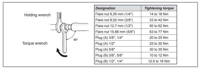
Figure 21 - Tightening torque
