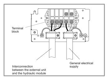
Figure 33 - Connections to outside unit's terminal block
