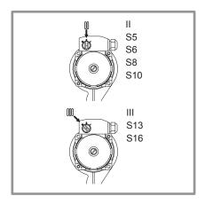
Figure 26 - Recommended circulation speed (for radiator)
