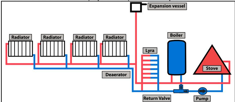
**Example scheme for installation of an anti-condensation valve. It is recommended that the valve be at least 50 C. At the discretion of the installer, a valve with a higher return water temperature may be installed.**
