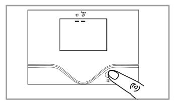
figure 11 - Selecting cooling mode
