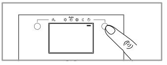
figure 12 - Selecting Frost protection mode
