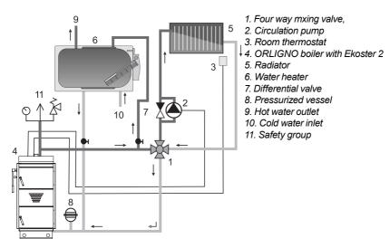
Pic.3 Connection scheme of ORLIGNO boiler with four way mixing valve and water heater.
