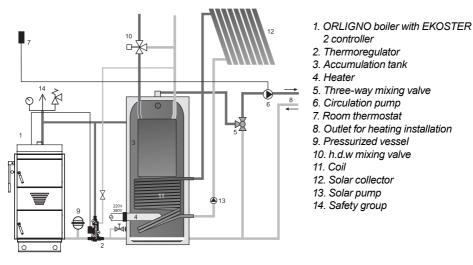
Pic.4 Connection scheme of accumulation tank type NADO with solar collectors.
