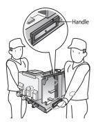
\* A minimum of two people should lift the unit by the handles and not by the drain pan or pipe work.
