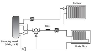
When two different zones are used with different temperatures, adjust the temperature of discharge water to high temperature water and control the amount of bypass to provide low temperature water by applying the mixing valve and temperature sensor of the mixing valve (TW4).
