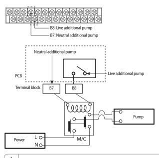
• The maximum allowable current that this terminal block can supply for the additional water pump is 0.1 A.
