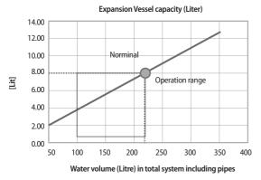
∴ Water volume of total system (except hydro unit) for reliable performance is minimum 20 liters (AE040/060/090RX\*\*).
