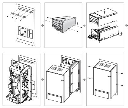
Fix screw through base panel of the unit.
