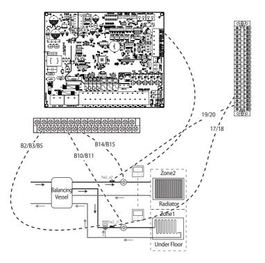
You can operate the 2-zone control using a mixing value, water-out temperature sensors, and built-in or external room temperature sensors installed in a wired remote controller.
