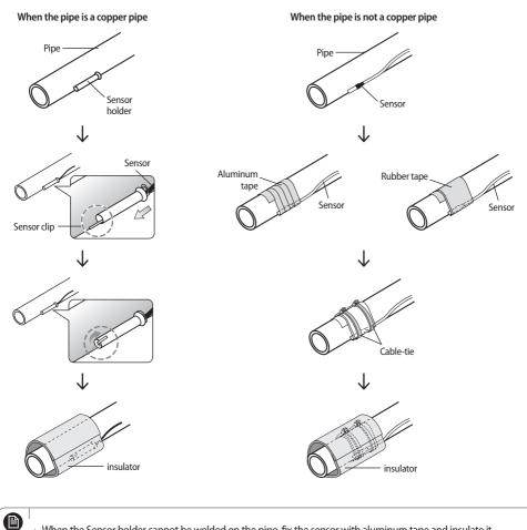
• When the Sensor holder cannot be welded on the pipe, fix the sensor with aluminum tape and insulate it.
