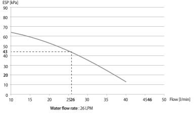
If the pressure loss of total system is over 43 kPa , additional water pump should be installed in series.
