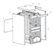
Two superior tie rods are screwed on three nuts at the front side of the boiler: the second and the third nut serve to place correctly the lateral sides of the casing. Two nuts, one for fixing the clamp holders for the lateral sides are screwed on the inferior tie rods, both form the front side and from the rear side. The assembly of the casing components has to be carried out in the following way:
