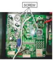
Remove the SCREWS and TRANSISTOR PCB.
