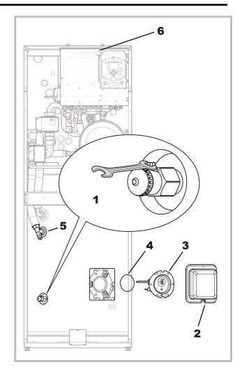
Figure 3 - Emptying the hydraulic unit and/or DHW tank
