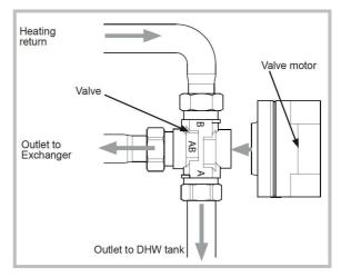
Figure 4 - Fitting the distribution valve
