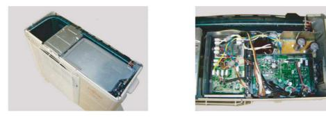
Remove the INVERTER BOX COVER by sliding upward.
