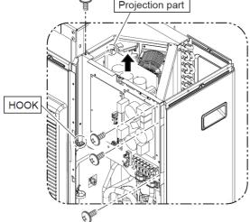
Remove the 4 mounting screws. Remove the PCB Case Assy upward.
