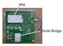
Spread SILICONE GREASE G746 evenly on the other side of the Diode Bridge and IPM when you exchange the Transistor PCB assy.
