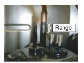
Cut the Discharge pipe in this range.
