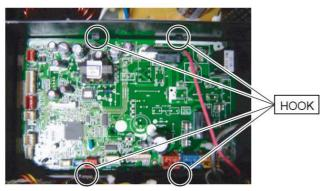
Remove the connectors and HOOK. Remove the MAIN PCB.
