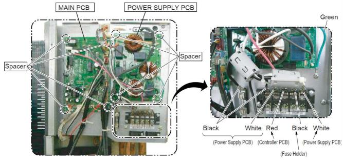
Remove the connector and cords. Remove the Spacer. Remove the MAIN PCB and POWER SUPPLY PCB.
