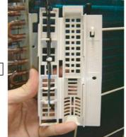
Open the THERMO HOLDER and remove the THERMISTOR.
