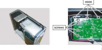
Remove the INVERTER BOX COVER by sliding upward.
