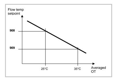
The cooling characteristic is adjusted for a 25°C room temperature setpoint. If the room temperature
