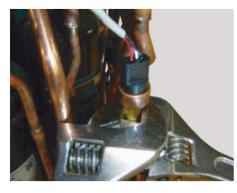
Remove the PRESSURE SENSOR with wrench. Note the tightening torque at the installation. Tightening torque is 12±1.5N•m.
