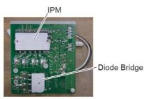
Spread SILICONE GREASE G746 evenly on the other side of the Diode Bridge and IPM when you exchange the Transistor PCB assy.
