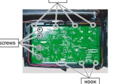
Remove the 4 mounting screw and hook. Remove the connectors and wires. Remove the MAIN PCB.
