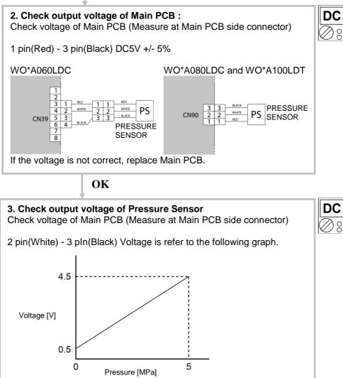
If the voltage is not correct, replace Presure Sensor.
