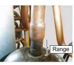
Cut the Suction pipe in this range. Remove the COMPRESSOR.
