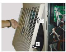
Remove the FAN GUARD by sliding upward.
