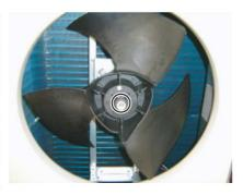
Remove the Hex Socket Screw. And remove the PROPELLER FAN. Note at the installation. Insert propeller Fan and Moter shaft reference D cutting position. And the tightening torque at the installation. Tightening torque is from 10 to 15N•m.
