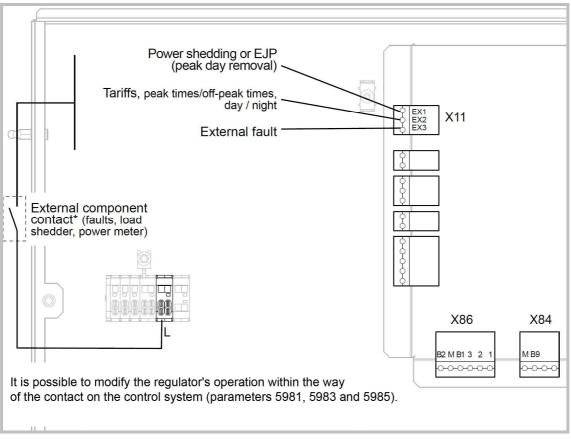
Figure 2: Typical Wiring of External Devices
