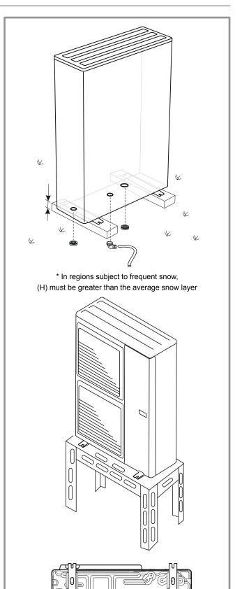
figure 12 - Positioning of the outside unit, draining away the condensate
