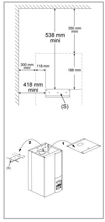
figure 13 - Mounting bracket
