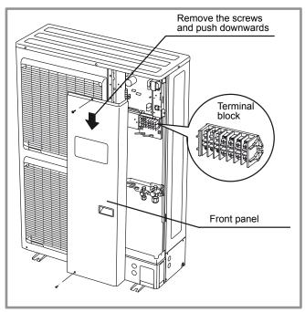
figure 27 - Access to 3-phase outdoor unit's terminal block
