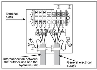
figure 28 - Connections to 3-phase outdoor unit's terminal block
