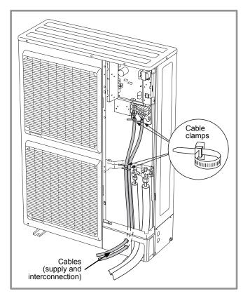
figure 29 - Finalisation of connection to 3-phase outdoor unit
