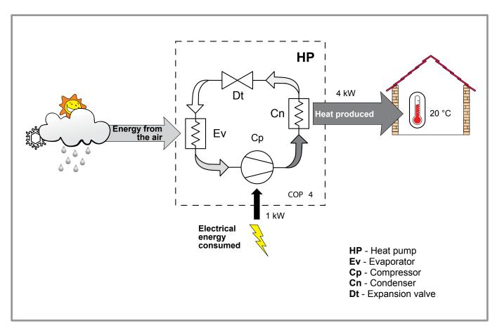
figure 8 - Heat pump operating principle
