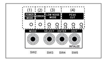
figure 46 - LED display on the 3-phase outdoor unit
