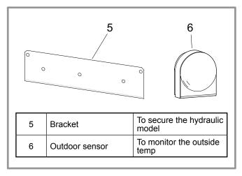
figure 10 - Accessories provided with the hydraulic unit
