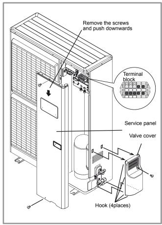
figure 24 - Access to sinlge phase outdoor unit's terminal block
