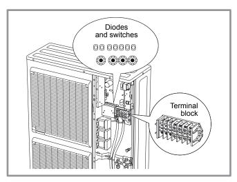
figure 45 - Location of switches and diodes on 3-phase outdoor unit
