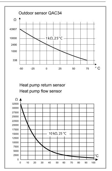
figure 4 - Ohmic values of the sensors (Hydraulic module)
