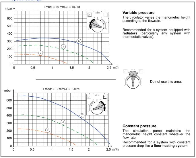
figure 22 - Hydraulic pressures and flow rates available
