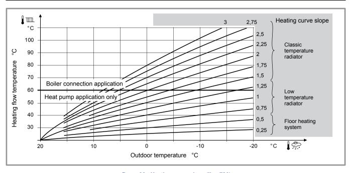
figure 36 - Heating curve slope (line 720)
