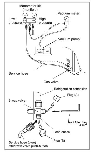
figure 17 - Extraction under vacuum and gassing
