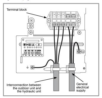
figure 25 - Connections to sinlge phase outdoor unit's terminal block
