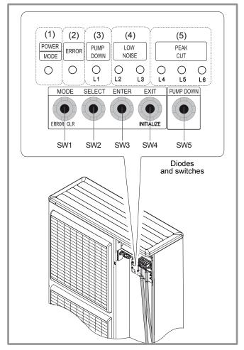
figure 44 - Location of switches and diodes on single phase outdoor unit
