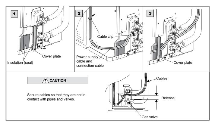
figure 26 - Finalisation of connection to sinlge phase outdoor unit
