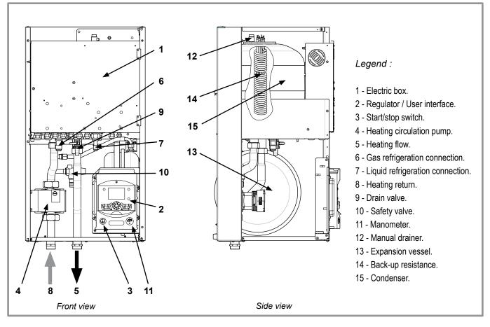
figure 7 - Hydraulic unit components
