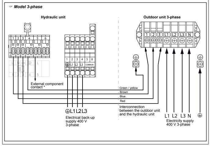
figure 33 - Connection to terminal block and power relays
