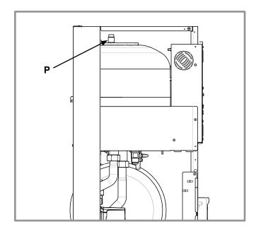
figure 20 - Hydraulic module bleeder valve
