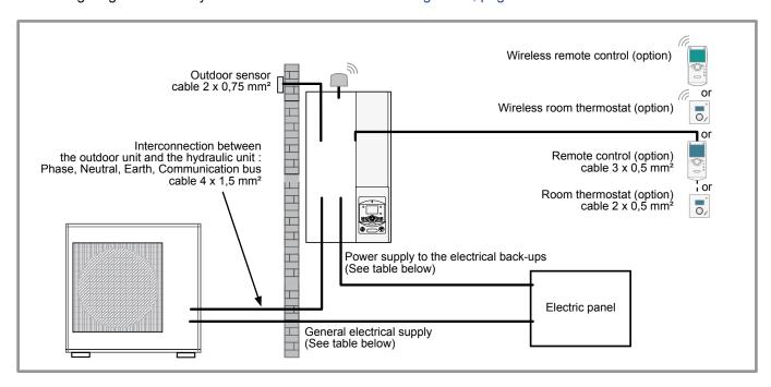
figure 23 - Overall layout of the electrical connections for a simple installation (1 heating circuit)
