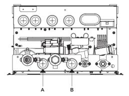
Hole A: for AC line (wire which is connected to the terminal block of the control box)
