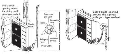
Trap is required to prevent water from entering into electrical parts.
