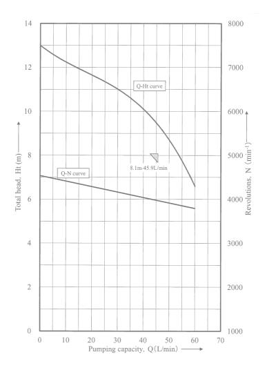
Performance test based on standard ISO 9906 with pre-pressure 2.0bar and liquid temperature 20°C.
