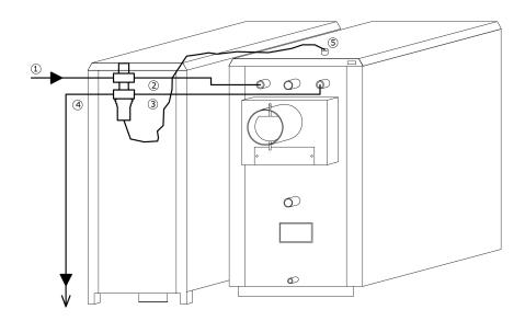
Connection scheme for the thermal safety valve: 1. Cold water entering from the water supply system 2. Cold water entry into boiler 3. Hot water going outside the boiler 4. hot water ending in the sewage water system 5. Thermo-valve sensor
