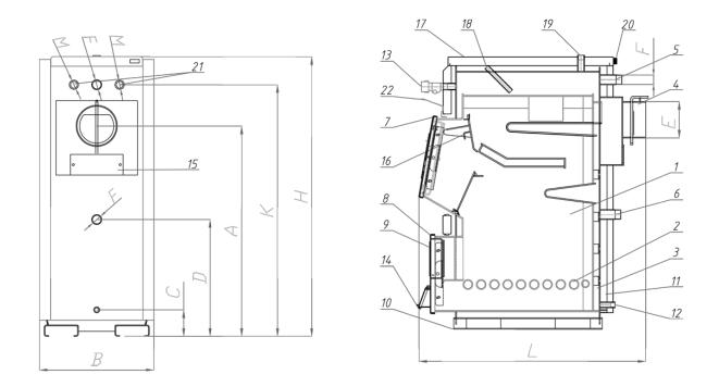
Parts of the boiler: 1. Combustion chamber 2. Grid 3. Boiler 4. Flue gas 5. Flow 6. Return 7. Upper door 8. Lower door 9. Burner mounting flange 10. Base 11. Insulation 12. Drain tap  $(\frac{1}{2})$  13. Draught regulator mounting place 14. Primary air flap 15. Opening for cleaning 16. Two/three pass flap 17. Housing 18. Thermostat against condensation 19. Safety pipe 20. Circulation pump connector 21. Thermal safety valve connection 22. Thermo-regulator protection
