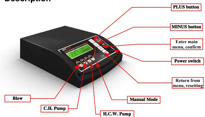
The **ST-32zPID** temperature regulator is intended for use with central heating boilers. The regulator is used for controlling the central heating water circulation pump, hot consumption water pump and blow (fan).
